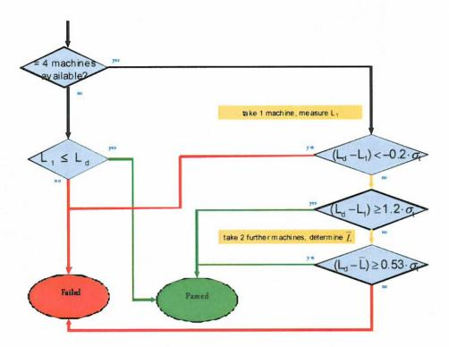
Figure 1: Verification procedure
