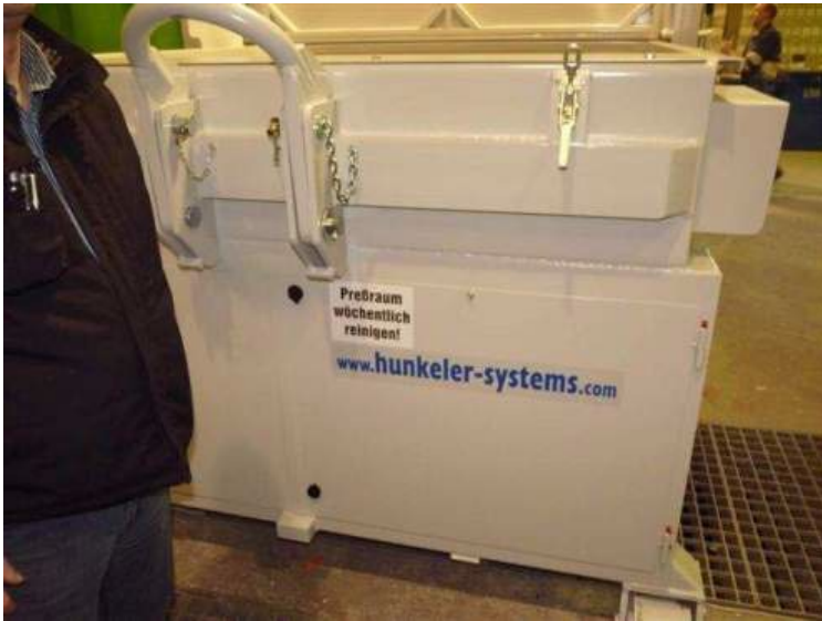
Figure: Maintenance door with instruction for weekly cleaning
